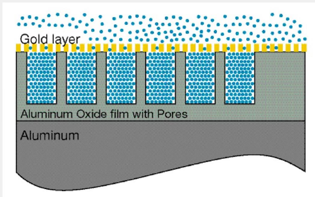
Operating Principle of Al<sub>2</sub>O<sub>3</sub> Sensor
