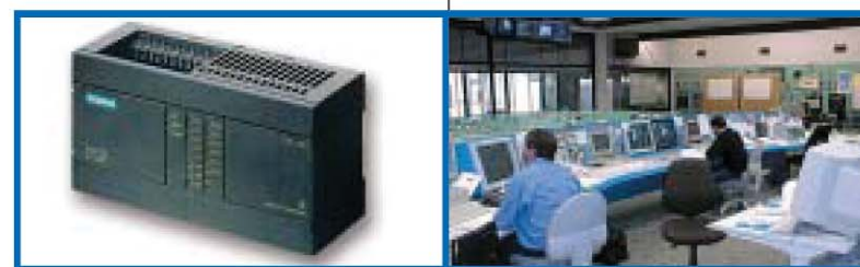
Alarm peaks are transferred to a PLC or a control room through 4-20 mA
