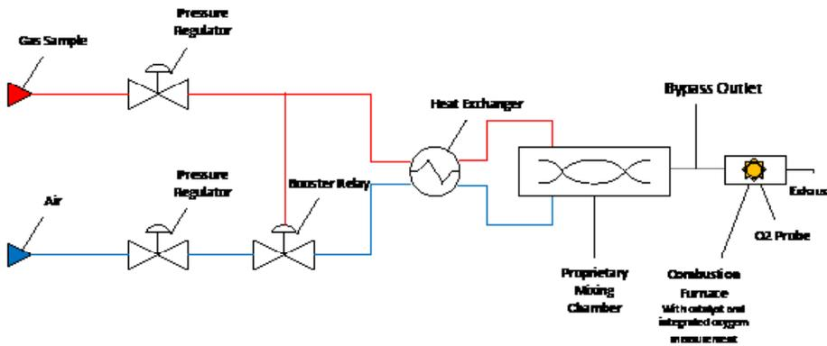
Pressure and temperature of gas sample and instrument air are equalized by means of pre-regulators, a dual chamber pressure exchange membrane regulator (booster relays) and a heat exchanger. The two streams then pass through precision orifices operating at super-critical stage through a proprietary low volume area mixing chamber. Orifice sizes are selected based on desired BTU range, precisely maintain a constant fuel-air ratio. The air-gas mixture then enters a combustion
