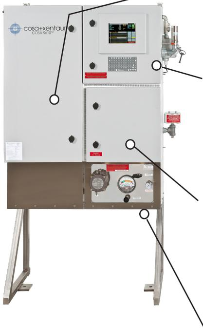
The **gas mixing compartment** contains sample conditioning and the gas mixing system. The gas mixing compartment is heated to avoid condensation of heavier gas constituents. All electrical components in the sample compartments are hazardous area rated.
