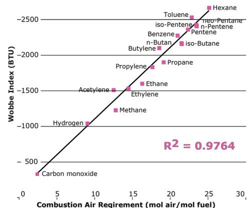
The table and graph above show the relationship of Wobbe Index and the Stoichiometric Dry Air Requirement for some typical gas constituents. The correlation is close to linear ( $R^2=0.9767$ ) with an intercept close to zero. The residual oxygen method takes advantage of this correlation by linear extrapolation between measurements of known calibration gases.  $R^2$  for typical natural gas constituents plus hydrogen and CO is 0.9888.
